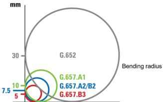
ITU recommendation G.657 specifies two classes of single-mode bend insensitive fiber patch cables: G.657 A and G.657 B. Each category (A and B) is then divided into two sub-categories: G.657.A1, G.657.A2 and G.657.B1, G.657.B2. The minimum bend radius of G.657.A1 fibers is 10 mm, of the G.657.A2 and G.657.B1 fibers is 7.5 mm and of the G.657.B2 fibers is 5 mm. Among, ITU-T G.657.A1 and ITU-T G.657.A2 fibers are fully compliant with ITU-T G.652.D fibers.
