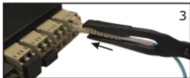
3. Grasp connector body with tool tips and gently push to ensure lock tab is engaged.
